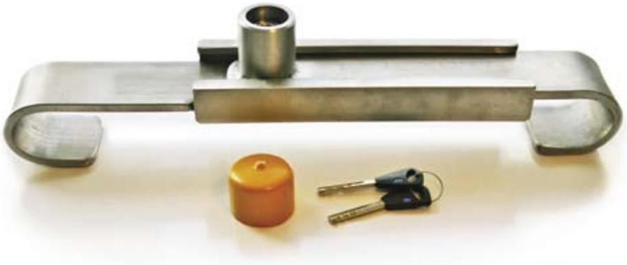
This lock is designed to provide additional security by clamping the vertical door closing rods in the closed position. It is constructed of 6mm thick hardened stainless steel and uses an Abloy lock to secure it.s
