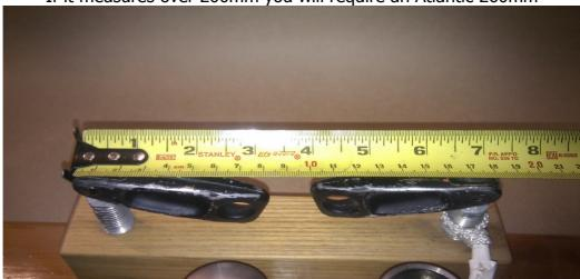
As shown in the example above 183mm will require an Atlantic Slot Lock 230mm
